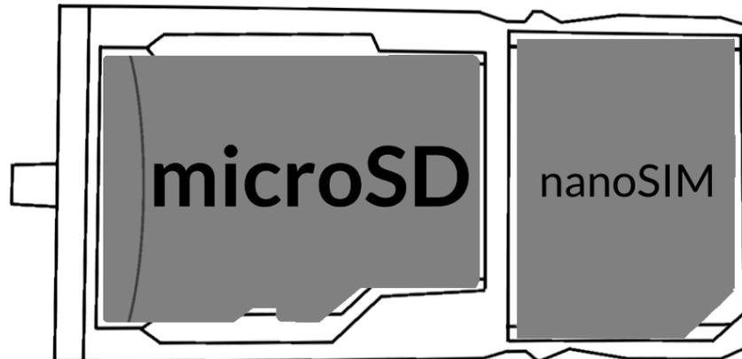
**⚠** Use only memory cards recommended by the manufacturer. Pay attention to the selection of the proper format-the microSD card, capacity and type / class. Incompatible memory cards may damage the device and cause the stored data to be destroyed as well. Incompatibility of memory card can be caused, among others, by an incorrect card format (required format microSD) or an unsupported card capacity - above the value recommended by the manufacturer.
